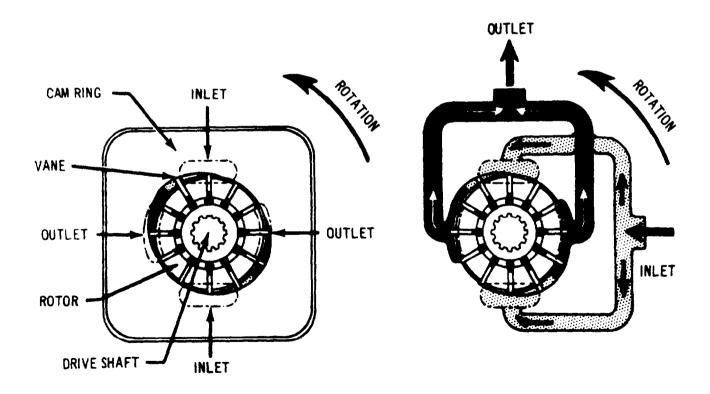
Figure 4B-2. Pump Cartridge Operation
