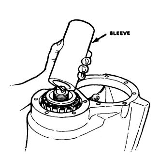
Figure 11-119. Pressing Bearing Cone with Sleeve
