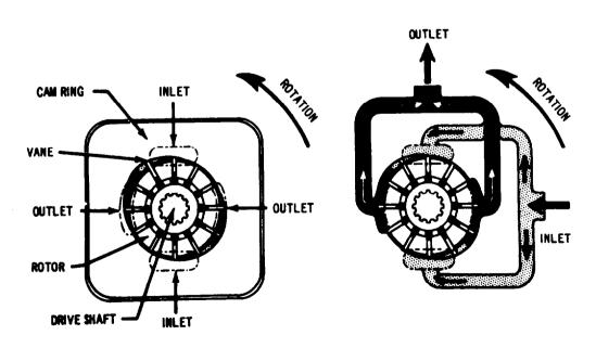
Figure 10-8. Hydraulic Pump and Pump Cartridge Operation
