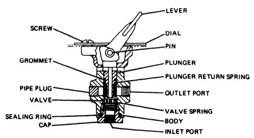
Figure 9C-11. Differential Lookout Valve (36Z1025)
