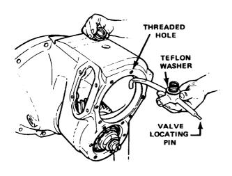
Figure 11-151. Installing Valve Body
