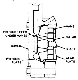
Figure 4B-26. Pressure Plate Operation
