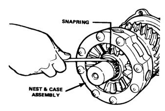
Figure 11-64. Nest and Case Assembly Removal
