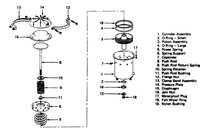
Figure 9D-5. Exploded View - Maxibrake Chamber
