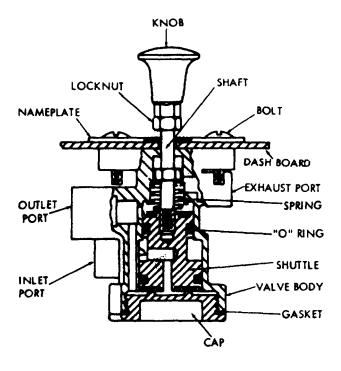
Figure 9C-8. Maxibrake Control Valve (36Z222)
