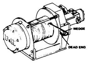
Figure 2-13. Securing Rope to Drum
