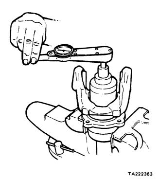
Figure 11-196. Reading Rotating Torque
