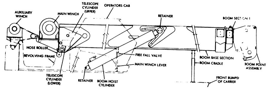
Figure 5A-1. Boom Installation (100J3482
