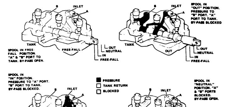
Figure 4D-11. Control Valve Operation (36Q70)
