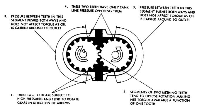
Figure 5K-6. Motor Operation
