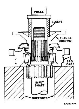
Figure 11-162. Yoke or Flange Installation
