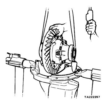
Figure 11-130. Installing Differential Assembly
