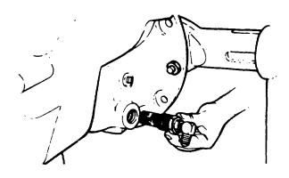
Figure 11-105. Tube Adapter and Related Parts
