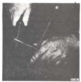
Figure 4D-16. Control Spool Disassembly
