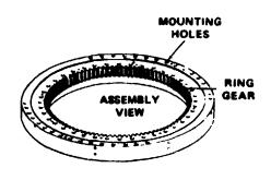
The slewing ring must be installed so that the word FRONT stamped on the inner race faces the reer of the cerrier. The word FRONT on the outer race must face the front of the upper.
