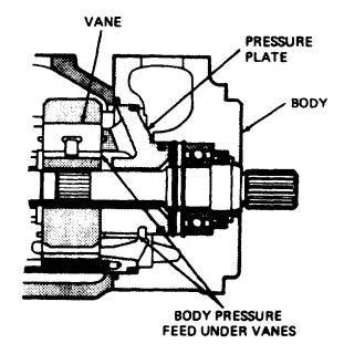
Figure 4B-17. Pressure Plate Operation
