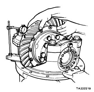
Figure 11-52. Measuring Gear Backlash
