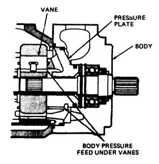
Figure 4B-39. Pressure Plate Operation
