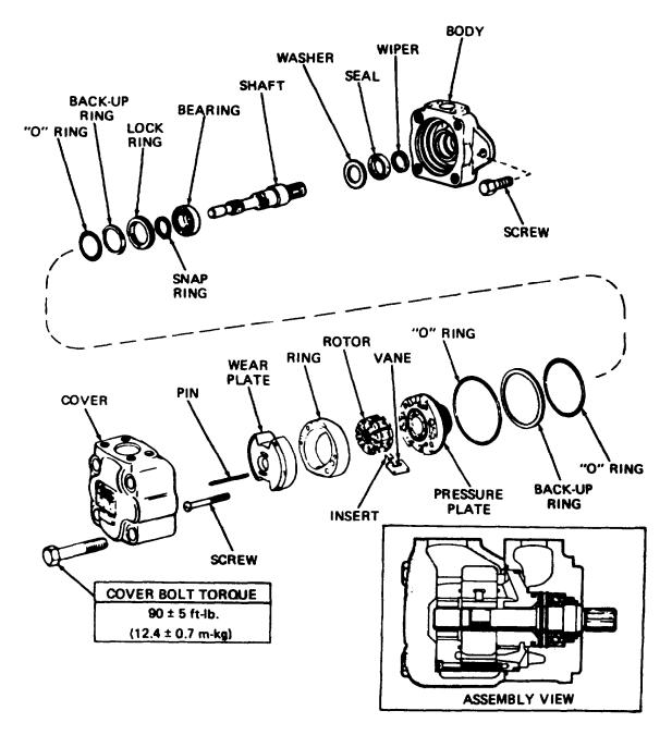
REASSEMBLY. Reassemble the pump, with a preassembled pumping cartridge, as follows:
