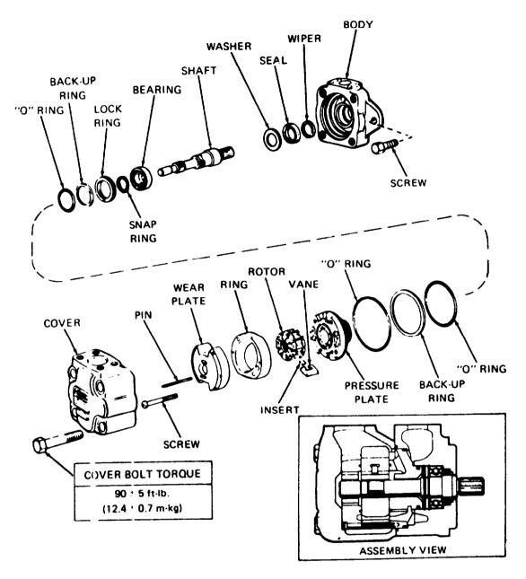
Figure 4B-18. Exploded View of Single Pump
