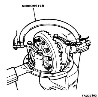
Figure 11-135. Measuring Carrier Leg Spread
