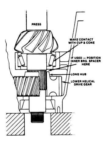
Figure 11-143. Installing Drive Pinion
