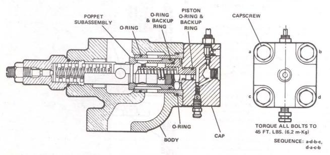
Figure 5F-6. Counterbalance Valve (36Z838)
