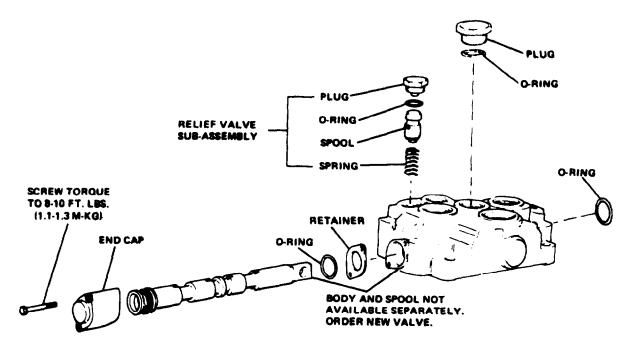
Figure 4D-4. Control Valve (36Z725)
