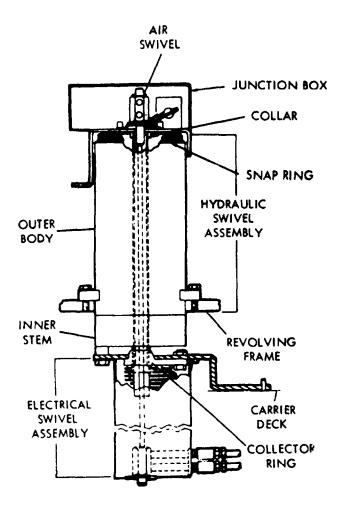
Figure 4C-2. Rotary Joint (979J30)
