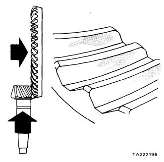
Figure 11-29. Incorrect Tooth Contact
