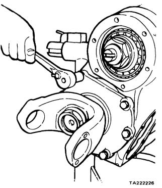
Figure 11-59. Input Shaft Bearing Cage Removal
