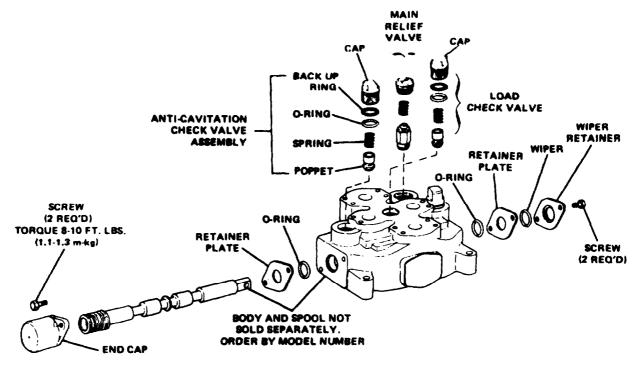
Figure 4D-8. Control Valve (36Z727)
