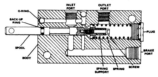
Figure 5H-3. Winch Brake Valve (36Z1028)
