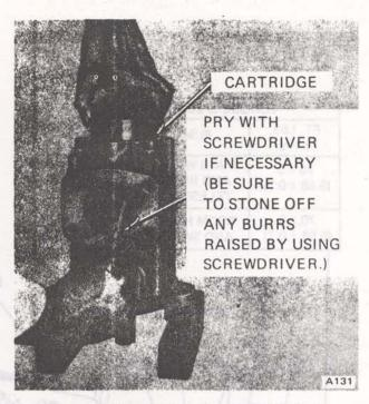
Figure 4B-30. Removing Cover End Cartridge
