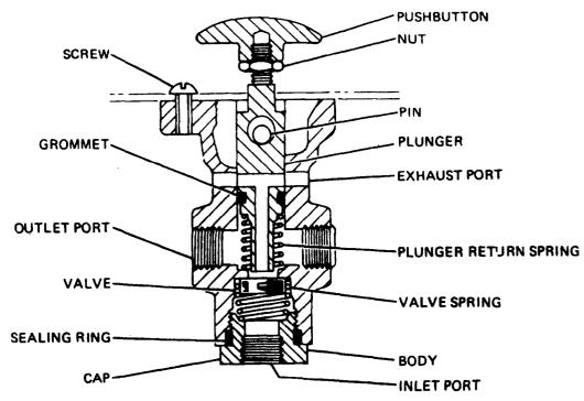
Figure 9C-10. Differential Lockout Valve (36Z289)
