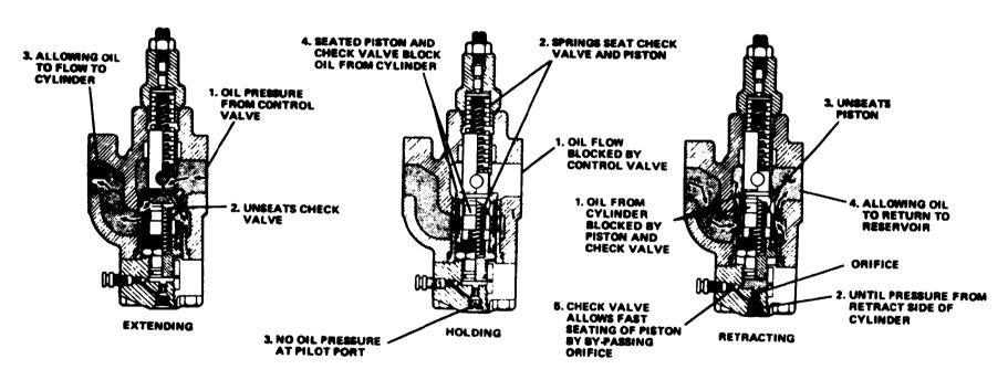
Figure 5F-1. Counterbalance Valve Operation (36Z683)
