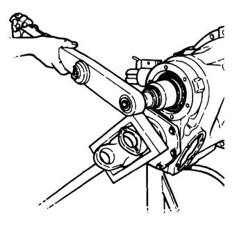
Figure 11-57. Pinion Nut Removal
