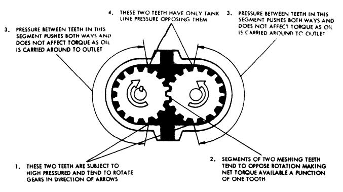
Figure 5K-2. Motor Operation
