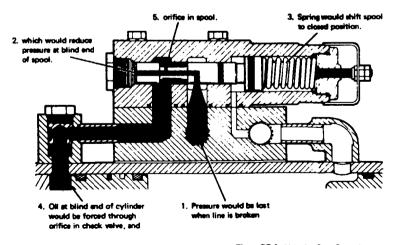
Figure SG-1. Velocity Fuse Operation
