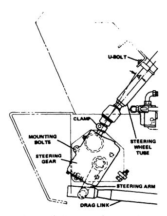
Figure 10-4. Steering Gear and Column Mounting
