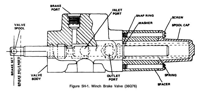
SUB-SECTION 5H WINCH BRAKE VALVES
