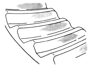
The pattern on the coast side of teeth will appear the same width as the drive side; however, the over-all length will be centered between the toe and heel of gear tooth.
