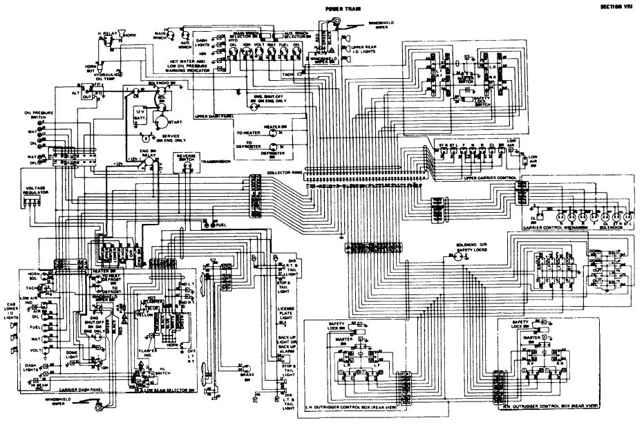
Figure 8-17. Carrier Electrical Schematic (100X139)
