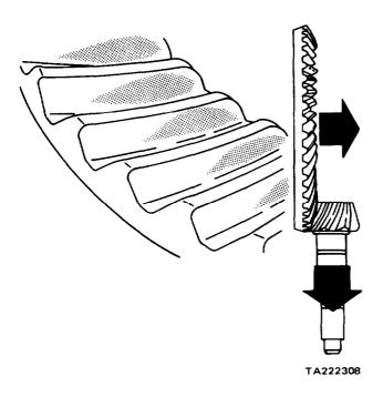
Figure 11-141. Low Pinion Contact
