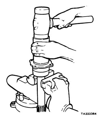
Figure 11-197. Tapping in Seal with Mallet
