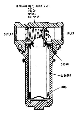
Figure 10-2. High Pressure Filter (46Z133)
