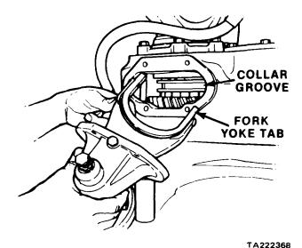
Figure 11-201. Installing Shift Unit Assembly
