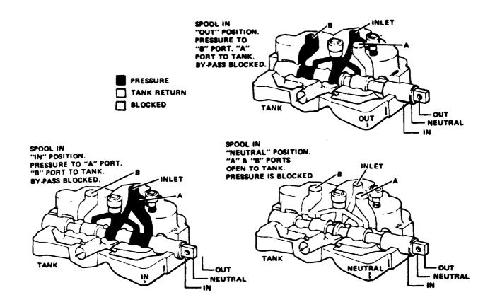
Figure 4D-5. Control Valve Operation (36Z726)
