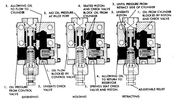
Figure 5F-7. Counterbalance Valve Operation
