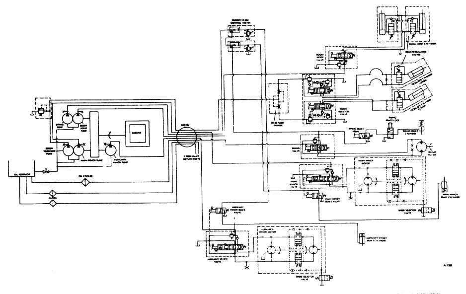
Figure 4A-5. Hydraulic Systems Schemetic (100X133-8).
