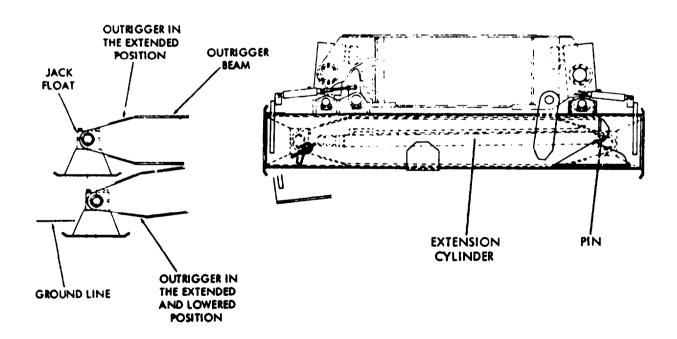
Figure 7-1. Hydraulic Outrigger Assembly
