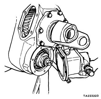
Figure 11-56. Carrier Pinion Cover Removal Current Model
