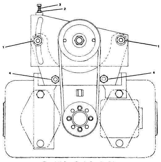
Figure 8-15. Power Steering Pump Installation
