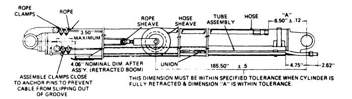
Figure 5C-2. Hose Loop Assembly (100J3870)
