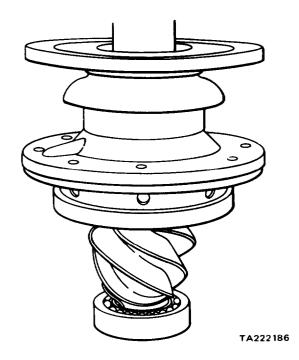
Figure 11-19. Installing Tapered Shaft Rear Bearing
