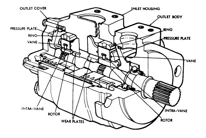
Figure 4B-23. Dual Pumps (41Z102 and 41Z103)
