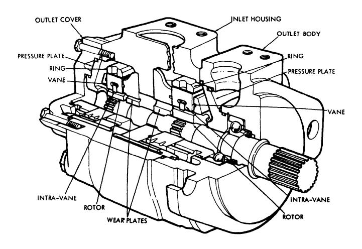
Figure 4B-1. Dual Pumps (41Z55 and 41Z56)
