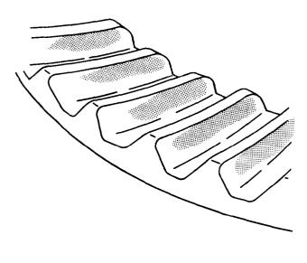
Figure 11-28. Satisfactory Tooth Contact (Gears Loaded)
