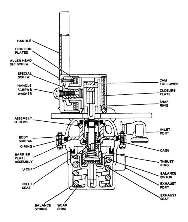
Figure 9C-17. Hand Throttle Valve (36U54)
