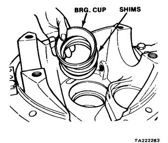
Figure 11-116. Bearing Cup and Shims
