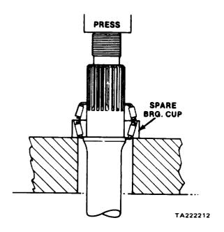
Figure 11-45. Press Method to Remove Bearing
