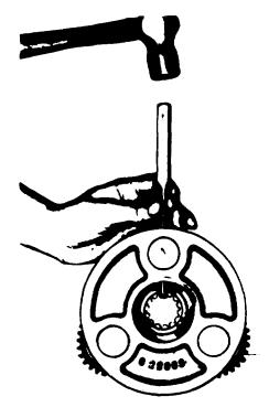
Figure 6B-4. Removing Planet Pins
