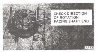
Figure 4B-10. Installing Rotor
