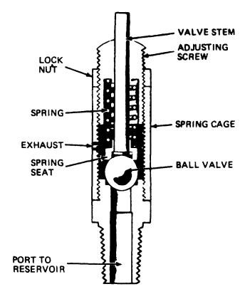
Figure 9C-2. Safety Valve (36Z6)
