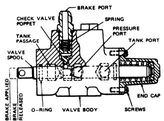
Figure 6F-1. Swing Brake Valve (36Q45)
