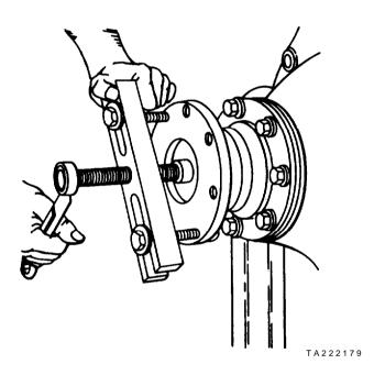
Figure 11-12. Carrier Flange Removal
