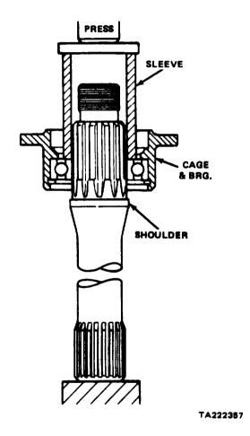
Figure 11-190. Installing Cage Assembly
