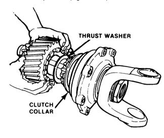
Figure 11-66. Removing Helical Drive Gear
