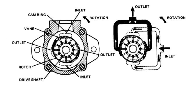
Figure 4B-24. Pump Cartridge Operation
