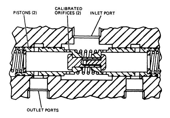
Figure 5D-1. Flow Divider Operation
