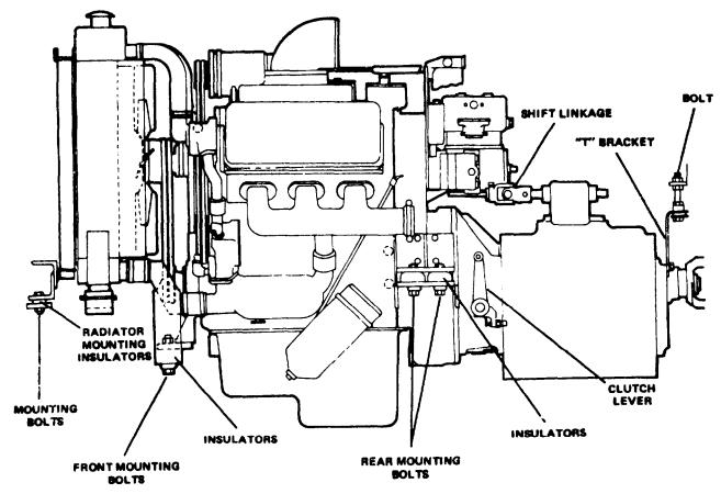
Figure 8-9. Engine and Transmission Mounting
