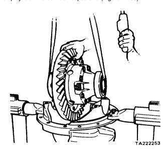
Figure 11-86. Removing Differential and Gear Assembly D. Using a suitable and safe lifting fixture, lift out the main differential and gear assembly from carrier (Figure 11-86).
