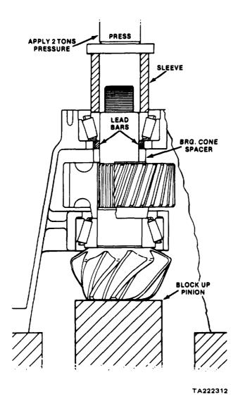
Figure 11-145. Setting Helical Gear Preload
