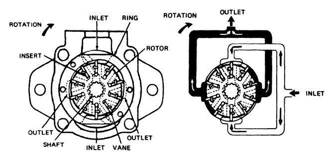
Figure 4B-37. Pump Cartridge Operation
