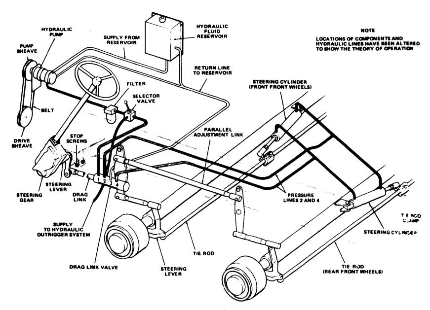
Figure 10-1. Steering System Schematic
