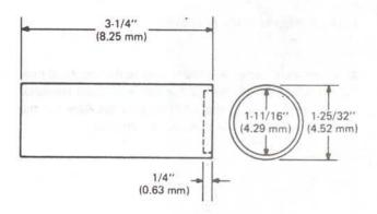
The driver can be made from tubular stock machined to the above dimensions.
