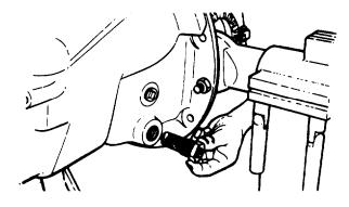
Figure 11-154. Installing Filter Screen Assembly
