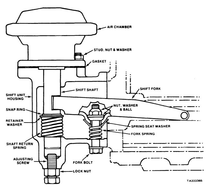
Figure 11-198. Inter-Axle Differential Shift Unit
