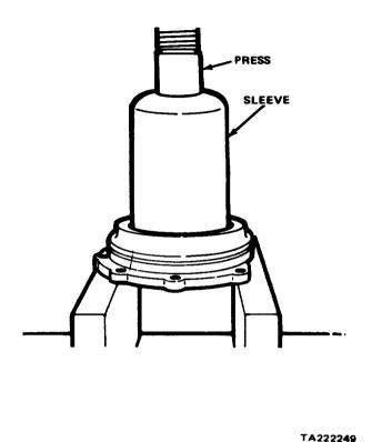
P. Remove the front or outer bearing retainer snapring from groove in inside diameter of the earlier one piece cages. Press out the oil seal with a suitable sleeve as shown above in Figure 11-82. Discard seal. With later models, press out oil seal from the input cage cover. If a press is not available use a drift and mallet to tap out seal. Be careful not to damage the cage or cover inside surface. Discard seal.
