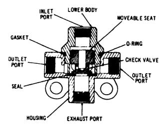
Figure 9C-7. Exhaust & Pressure Retaining Valve (36Z221)
