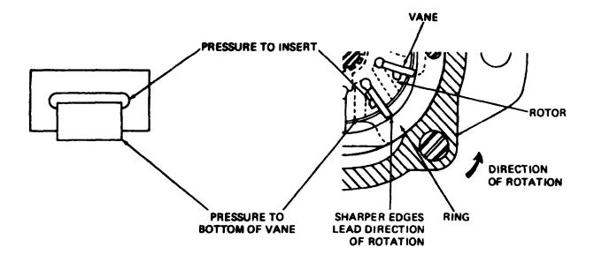
Figure 4B-25. Pressure Feed to Vanes
