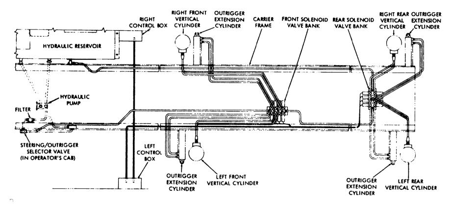
Figure 7-2. Hydraulic Outrigger Control System (8100J3980)
