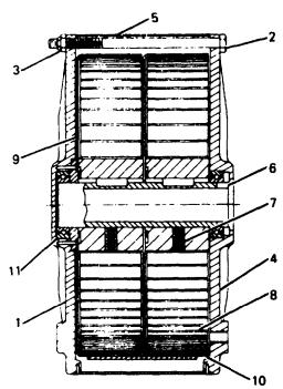
Figure 5E-2. Hose Reel Spring Motor
