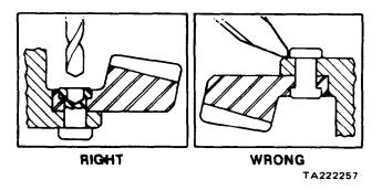
Figure 11-90. Drilling Out Rivets
