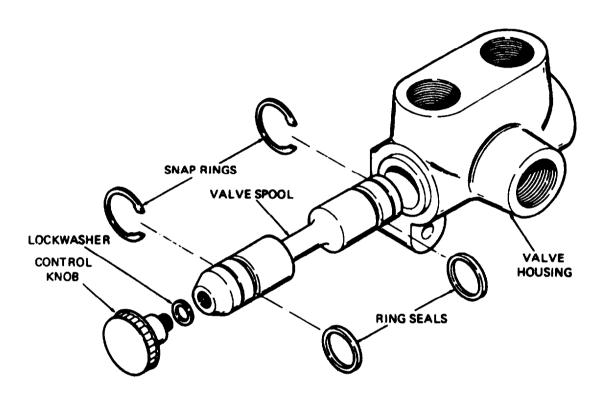
Figure 6G-1. Swing Brake Lock Valve (36Z361)
