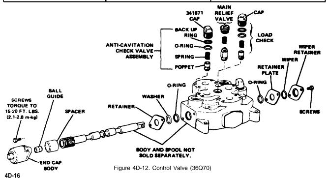
1. Discard all old O-rings and back up rings. Wash all parts in a clean mineral oil solvent and place them on a clean surface for inspection.
