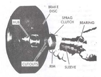
Figure 5J-18. Installing Sprag Clutch
