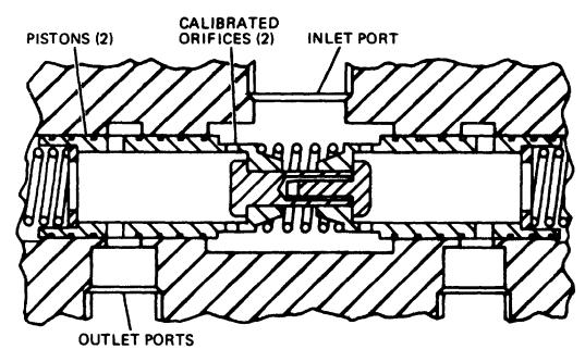
Figure 5D-3. Flow Divider Operation
