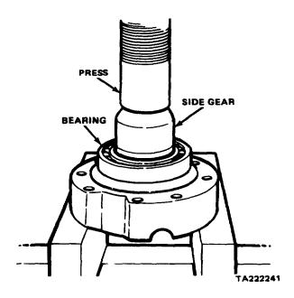
Figure 11-74. Side Gear Removal
