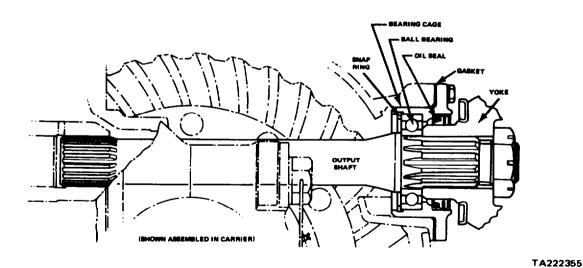
Figure 11-188. Output Shaft and Bearing Cage Assembly (Original Model)
