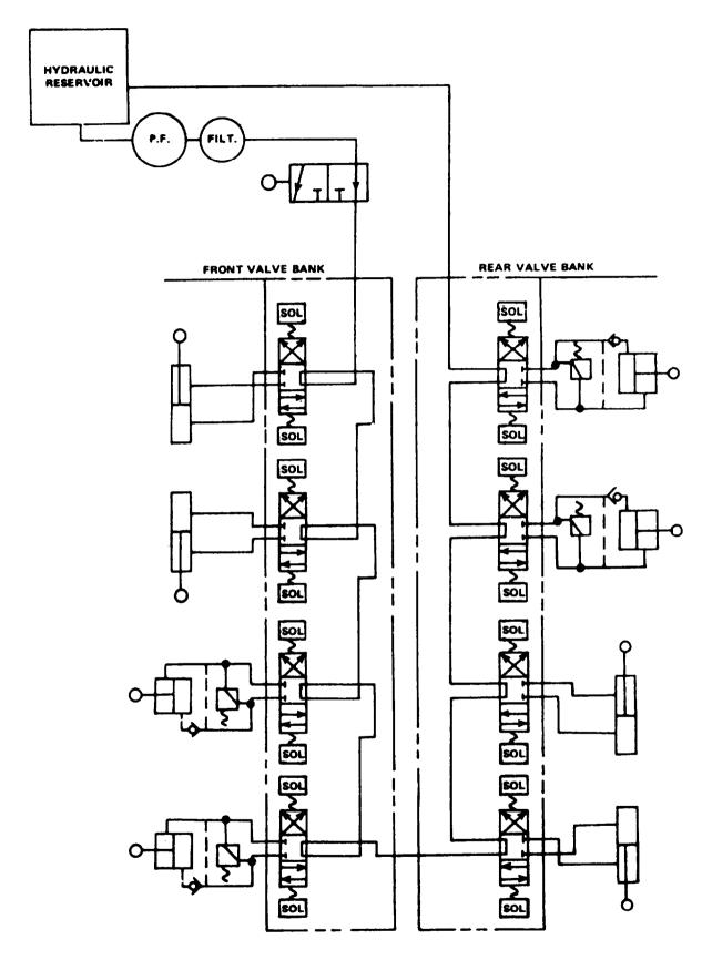
Figure 7-3. Outrigger Hydraulic Schematic (8100J3980)
