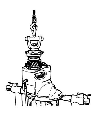
Figure 11-178. Axle on Lifting Fixture
