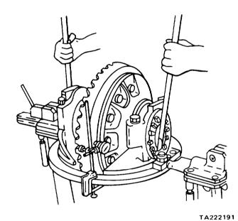
Figure 11-24. Adjusting Differential Bearing Preload
