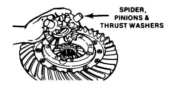
Figure 11-123. Installing Spider with Pinions
