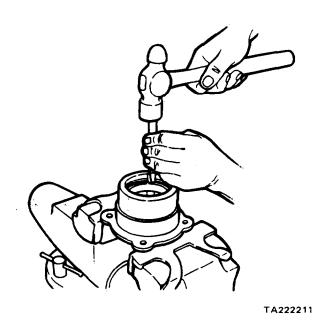
Figure 11-44. Inner Bearing Cup Removal
