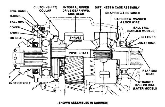
Figure 11-168. Ball and Straight Roller Bearings (Original Models)
