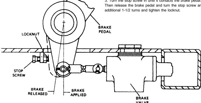
Figure 6F-2. Brake Pedal Stop Adjustment (100J4194-1-A)
