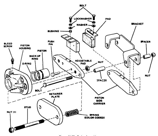
Figure 5J-23. Brake Assembly
