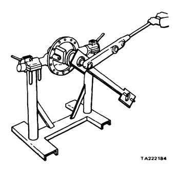
Figure 11-17. Torquing Pinion Shaft Nut
