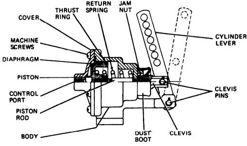
Figure 9C-14. Throttle Cylinder (36U30)
