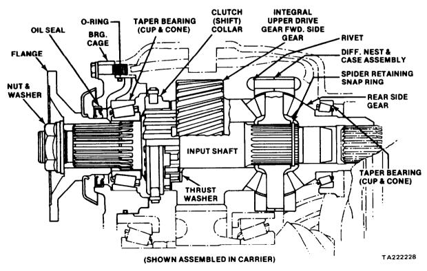
Figure 11-61. Inter-Axle Differential Assembly
