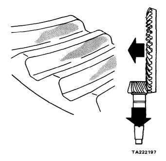
Figure 11-30. Correcting Pinion Depth
