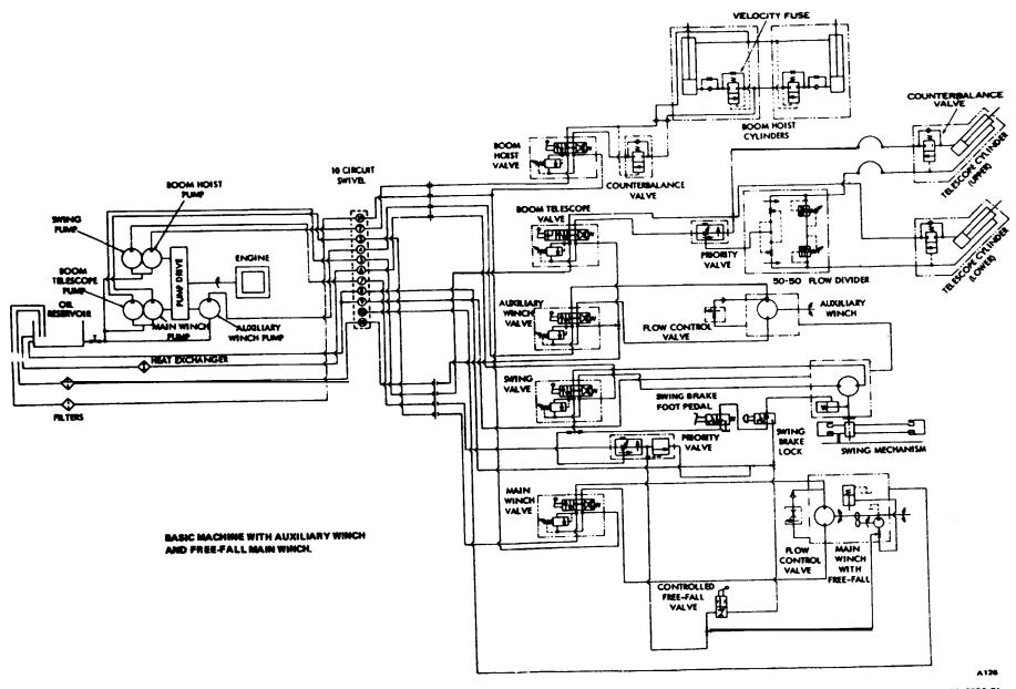
Figure 4A-3. Hydraulic System Schematic (100.03556-G)
