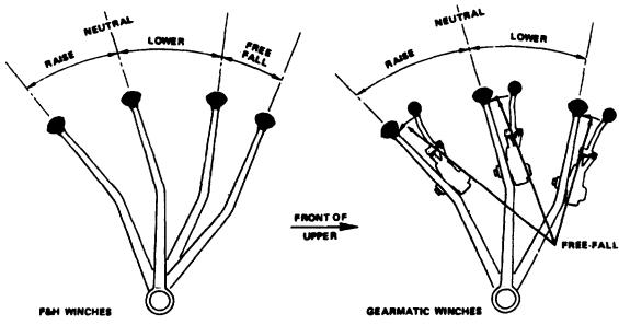
Figure 2-8. Winch Lever Positions
