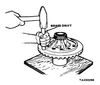
Figure 11-92. Gear Removal from Case
