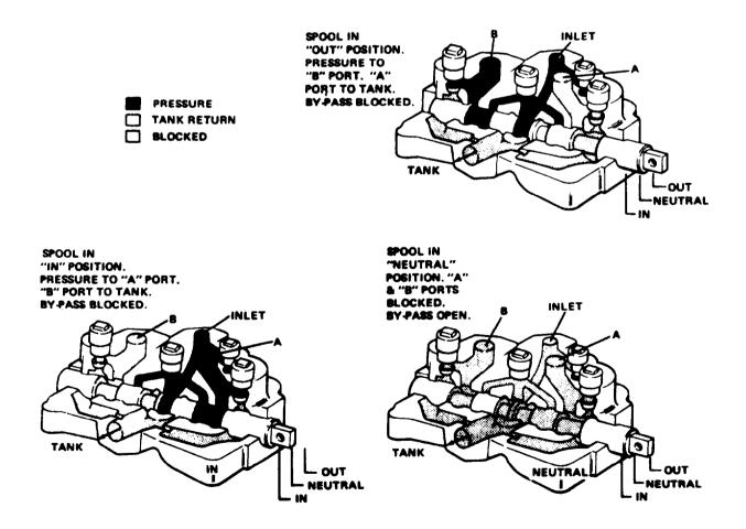
Figure 4D-7. Control Valve Operation (36Z727)
