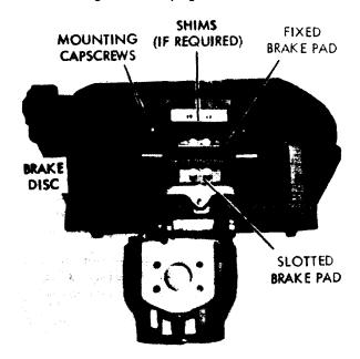
Figure 5J-21. Winch Brake Assembly
