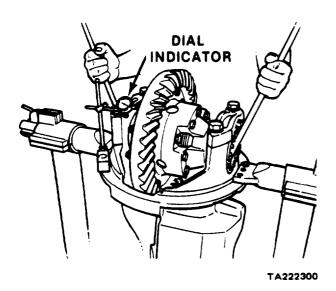
Figure 11-133. Preloading Differential Bearings
