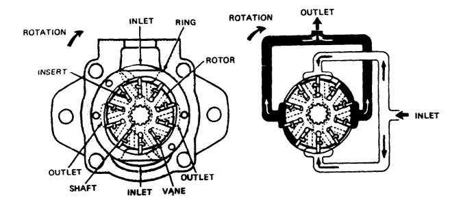
Figure 4B-15. Pump Cartridge Operation
