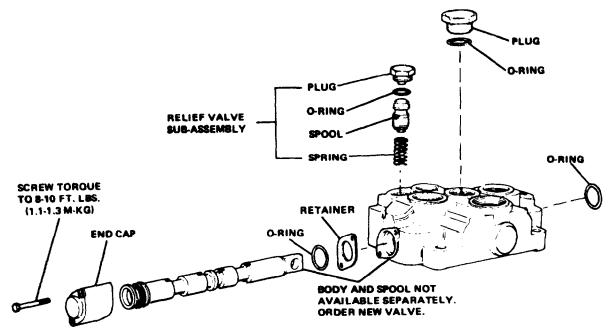
Figure 4D-2. Control Valve (36Z724)
