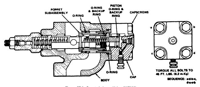
Figure 5F-3. Counterbalance Valve (36Z683)
