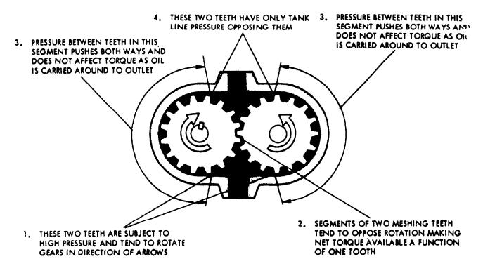
Figure 6C-1. Swing Motor Operation
