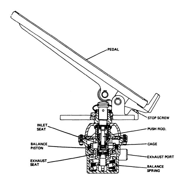
Figure 9C-15. Throttle Valve (36U29)
