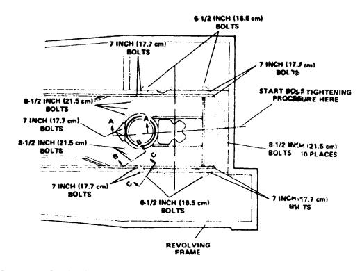
Figure 6E-1. Slewing Ring Installation (100J3517)
