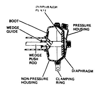
Figure 9D-2. Brake Chamber (1038Z170)
