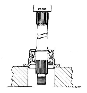
Figure 11-43. Installing Cage on Output Shaft
