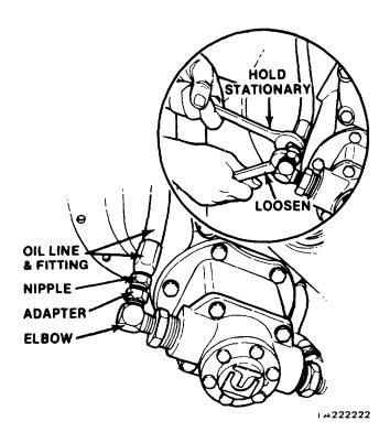
Figure 11-55. Disconnecting Oil Lines
