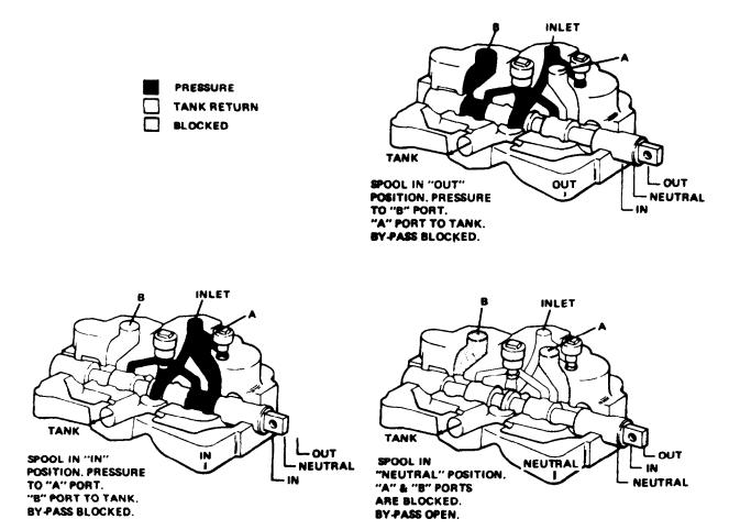
Figure 4D-9. Control Valve Operation (36Z986)
