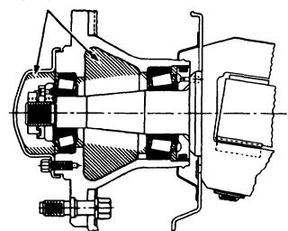
THE SHADING IN EACH INDICATES THE RECOMMENDATION FOR THE CORRECT AMOUNT OF GREASE.
