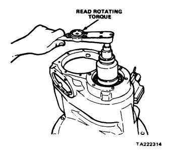
Figure 11-147. Checking Pinion Bearing Preload
