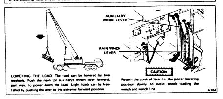
Figure 2-9. Crane Operating Cycle - P&H Winch
