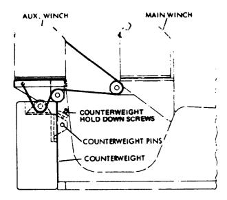
Figure 2-19. Counterweight Removal (1002382)
