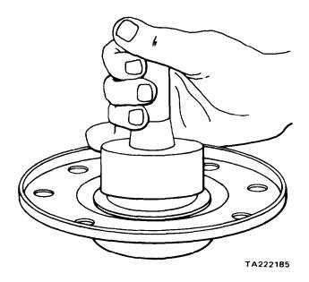
Figure 11-18. Installing Pinion Shaft Seal
