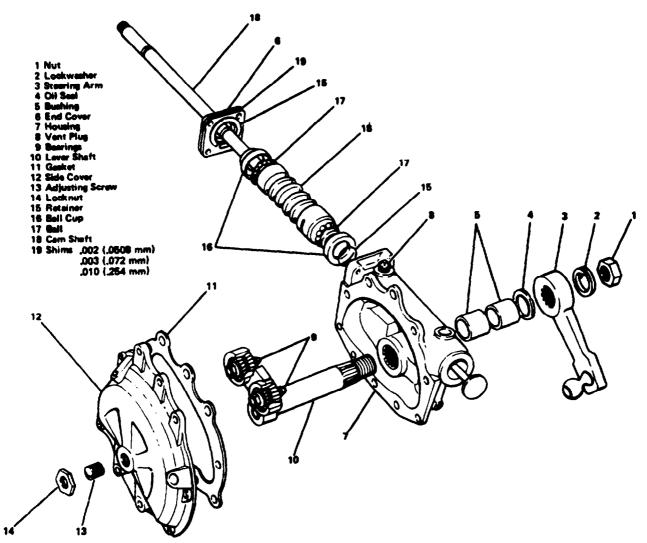
Figure 10-6. Steering Gear (53Z341)
