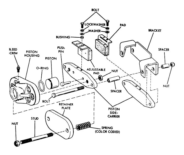
Figure 22. Brake Assembly
