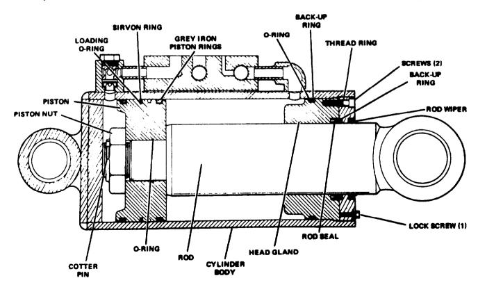
Figure 5B-1. Boom Hoist Cylinder (38Z231)
