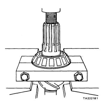
Figure 11-14. Pinion Shaft Bearing Removal
