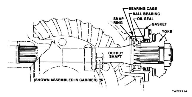
Figure 11-47. Original Model - Ball Bearing Assembly
