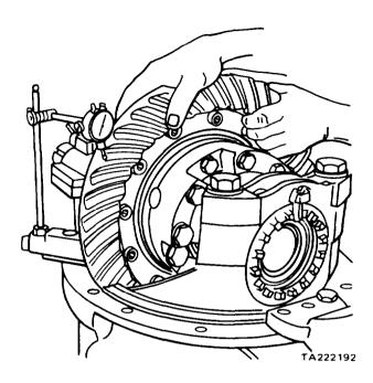
Figure 11-25. Checking Gear Backlash
