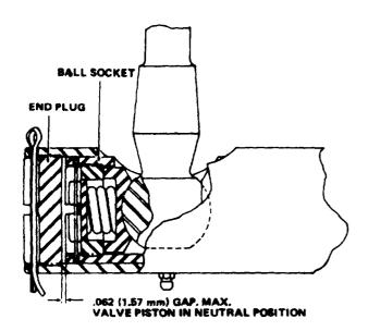
Figure 10-14. Adjusting End Plug Gap
