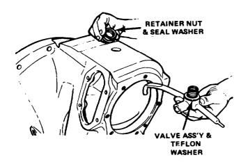
D. Disassemble the oil valve (pressure relief) only if required. Use the following procedure. Remove the retainer snapring from valve body opening and remove the washer, spring and ball (Figure 11-103).
