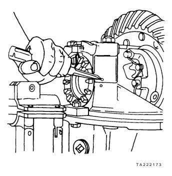
Figure 11-6. Center Punch Carrier Legend Bearing Cap
