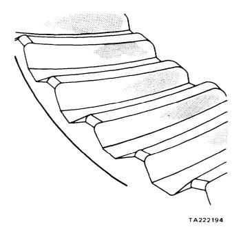
Figure 11-27. Satisfactory Tooth Contact (Gears Unloaded)
