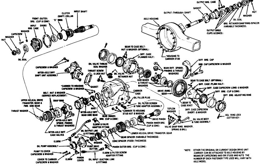
Figure 11-36. Current Design with Externally Mounted Oil Pump
