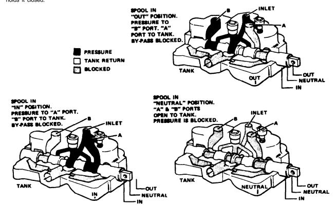
Figure 4D-1. Control Valve Operation (36Z724)
